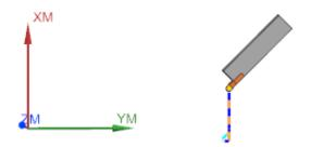
In this case, we need to output the spindle angle as "M66 BA=45.0 G52". In NX, we could set the BA angle in 2 places:
